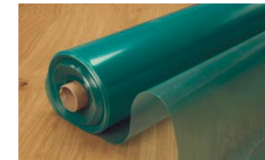
PE film (polyethylene) PGUDLSCREEN34, 12.5 x 2.7 m = 33.75 m² / roll Film that protects flooring from moisture vapour rising up from a mineral or concrete subfloor. Useful lifetime 50 years. Thickness: 0.2 mm. Material: Polyethylene, alkaline resistant.
